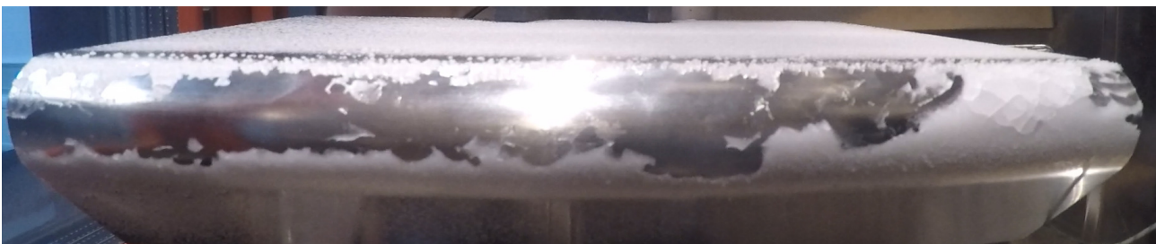
Figure 1: Picture of aerofoil showing the results of the piezoelectric based IPS.
