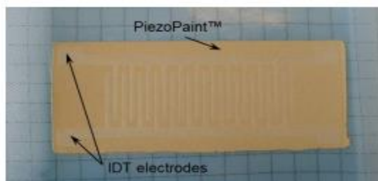
PiezoPaint™ based motion sensor printed directly onto the lab coat (Polycotton)
