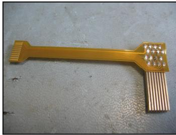
Fig. 7. Integration of the flex PCB on a piezo-composite sample.
