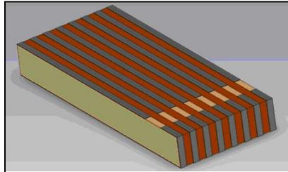
Fig. 2. Schematic view of a piezo-composite patch featuring 8 elements.
