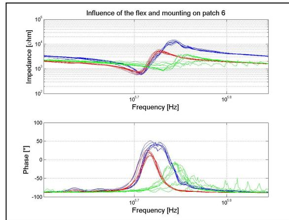
Fig. 9. Impedance of the patch n°5 before and after integration. Blue curves before integration, red curves after placing the flex PCB, green curves after integration completed.
