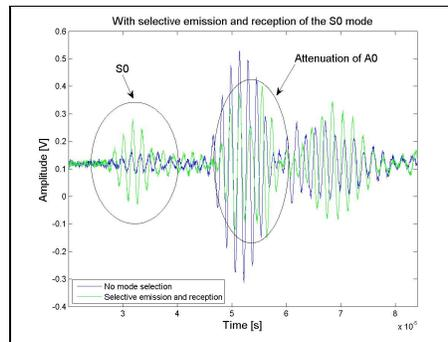
Fig. 17. Performance of the mode and direction selection techniques with  $S_0$  mode.
