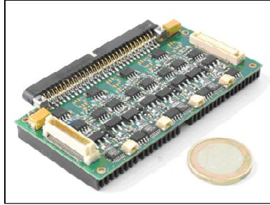
Fig. 12. 4-channels PULSECHO amplifier. Daughter board or embedded board.
