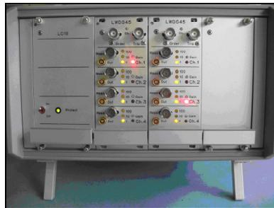
Fig. 10. Picture of a rack with two LWDS45-2 modules, i.e. multi-channel drive and sense electronics for piezo-patches.
