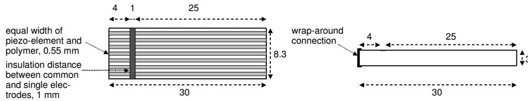
Fig. 4. Schematic representation of the the piezo-array patch, top view (left) and side view (right). All dimension are in millimeters. The common electrode on the bottom side is connected to the top side with a wrap-around connection.
