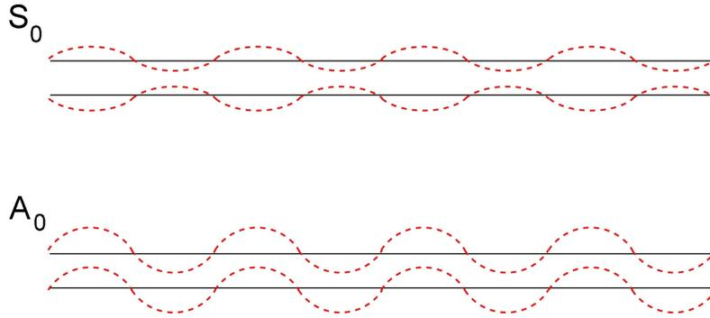
Fig. 1. Lamb waves in a thin plate: symmetrical  $S_0$  and antisymmetrical  $A_0$ .
