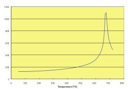
Free dielectric constant for Pz46 as a function of temperature. The Curie point is above  $650^{\circ}\text{C}$
